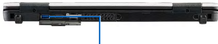
USB to Ethernet adapter port on the back of the laptop
