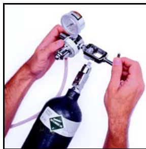
CO 2 Regulator Connected
