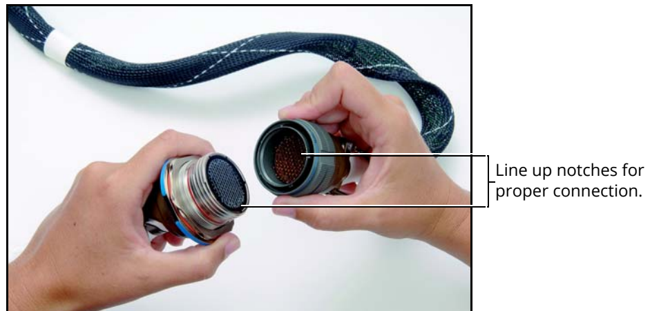
Electrical Connection to Umbilical
