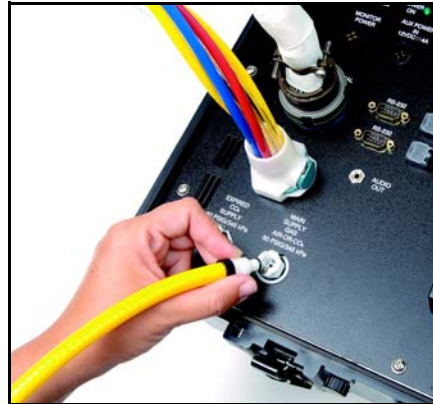
Connecting Air or CO 2 to the PCU
