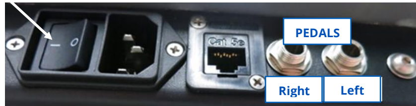
Main simulator power switch
