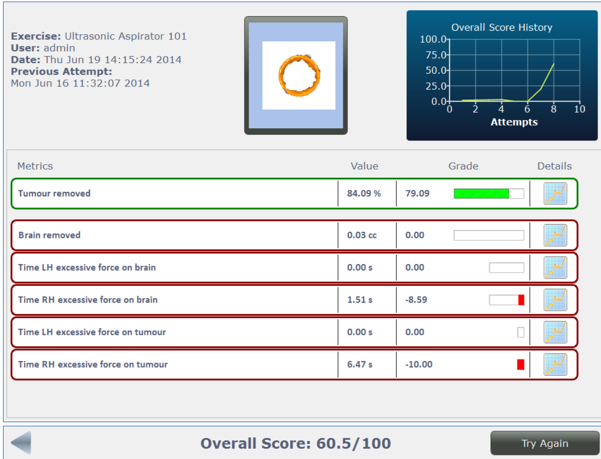
Figure 6: Tailored metrics and score for the Ultrasonic Aspirator 101 exercise. The exercise goal (outcome) appears at the top, outlined in green. Potential errors are listed below the goal and outlined in red. Grades for every metric value achieved are shown as both a number and a bar graph, where the length of bar indicates the maximum magnitude attainable. The overall score (out of 100) is the sum of all metric grades.
