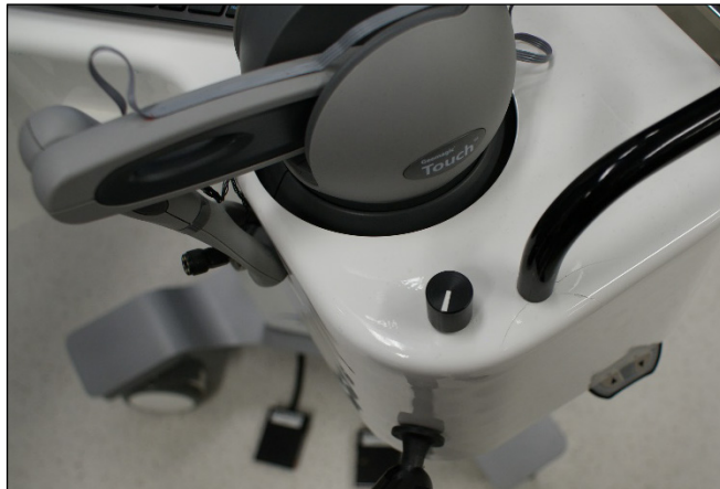
Power knob on workstation; intensity gauge depicted in simulator
