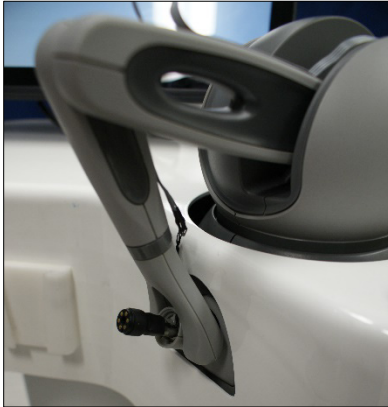
Haptic device tip inserted into inkwell during calibration procedure
