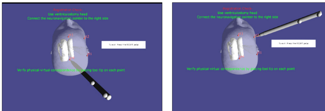
Checking head flap registration accuracy at various points
