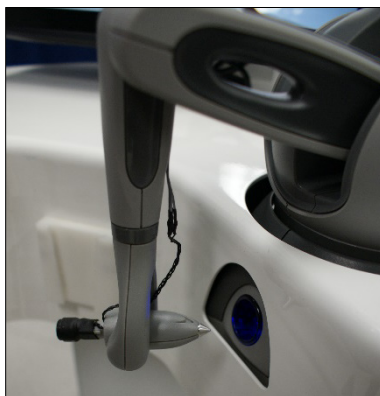
Haptic device tip outside of inkwell for start of calibration procedure
