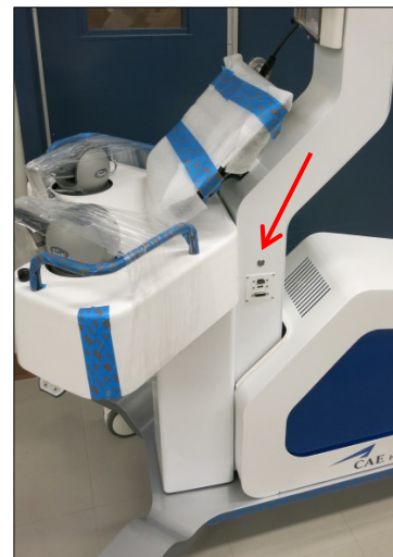
“On switch” at the back of simulator (left) and on side column (right)
