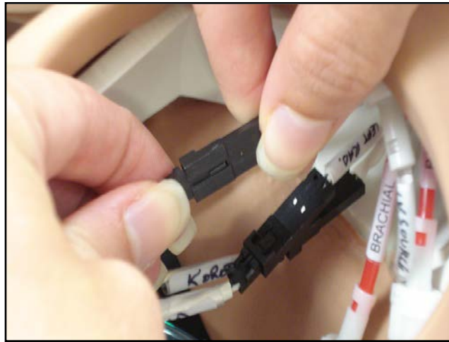
Disconnecting the Electrical Connectors
