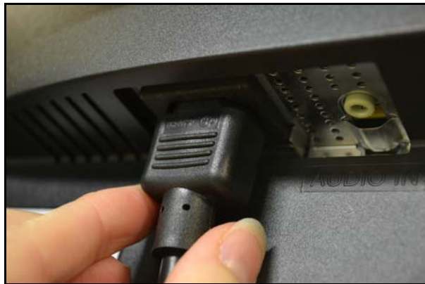
The Power Cable Connection
