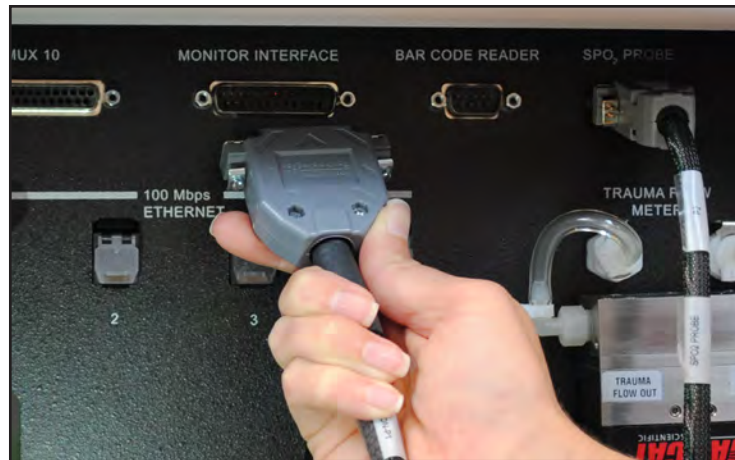
Connecting the Monitor Interface to the Back of the Rack
