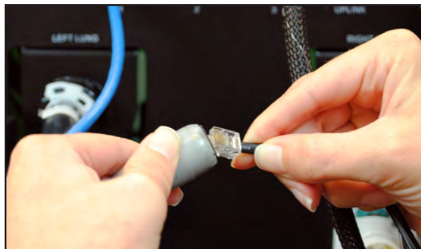
Connecting Standard Monitor Cables to the Monitor Interface
