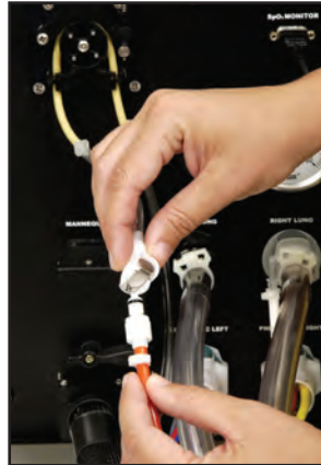
Attaching the GU Hose
