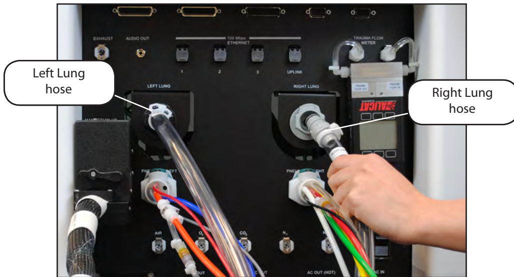
Attaching the Left Lung and Right Lung Hoses
