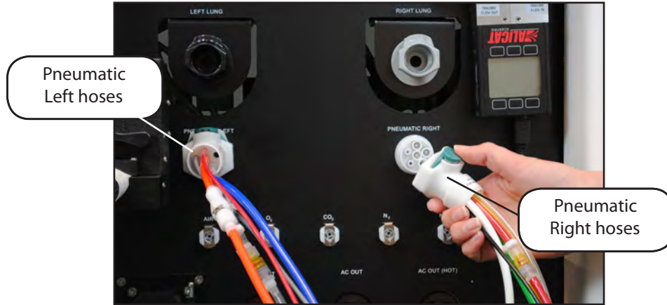
Attaching the Pneumatic Left and Pneumatic Right Hoses
