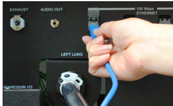
Connecting the Ethernet Cable to the HPS Lab Rack
