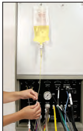
Connecting the Peristaltic Tubing to the IV Bag
