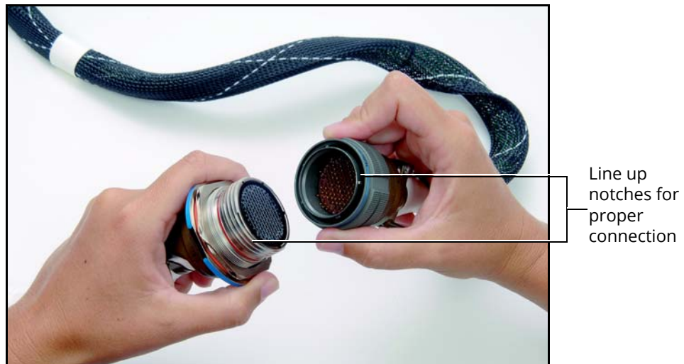
Electrical Connection to Umbilical
