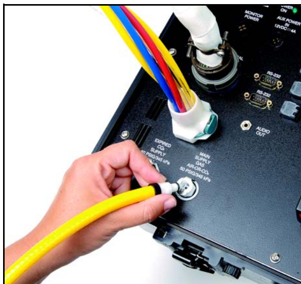
Connecting Air or CO 2 to the PCU
