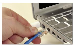
**Connect the Ethernet Cable to the Workstation**
