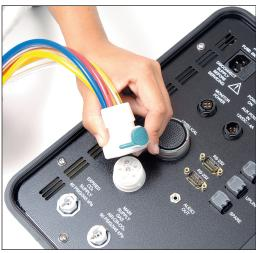
Fluidic/Pneumatic Coupler Connected to PCU
