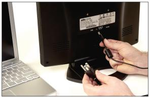
Plug the AC Cable into the Waveform Display Monitor
