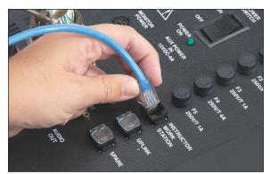
**Connect the Ethernet Cable to the PCU**
