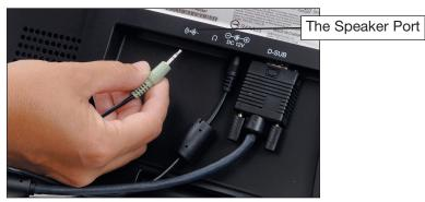
**Connect the Audio Cable to the Monitor**
