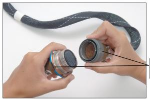
Line up notches for proper connection.
