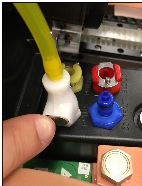
The Mannequin's Torso - Rotation Ring Compressor Connection
