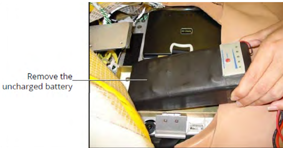
Removing the Battery Tie-Down
