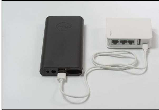
Router Plugged Into Battery Pack
