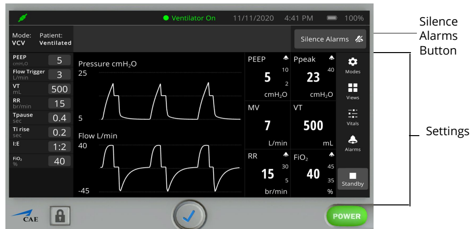
Transport Ventilator Screen - Ventilator On
