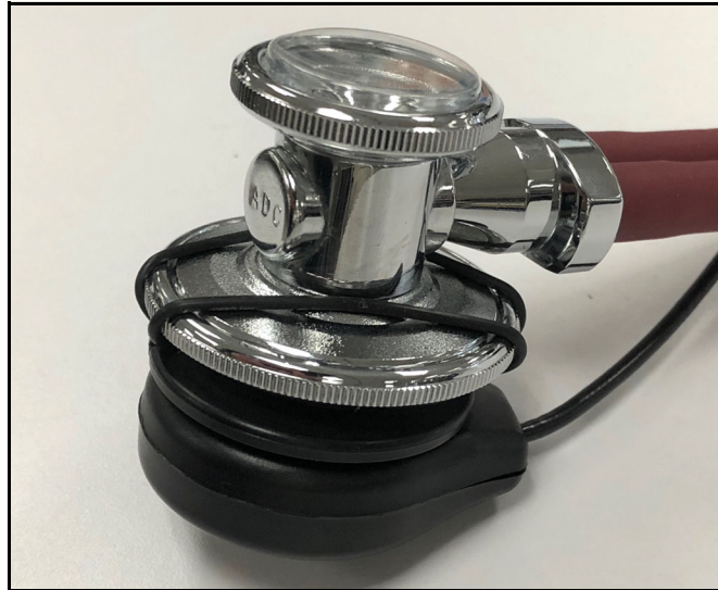
StethoSym Speaker Module Connected to Diaphragm
