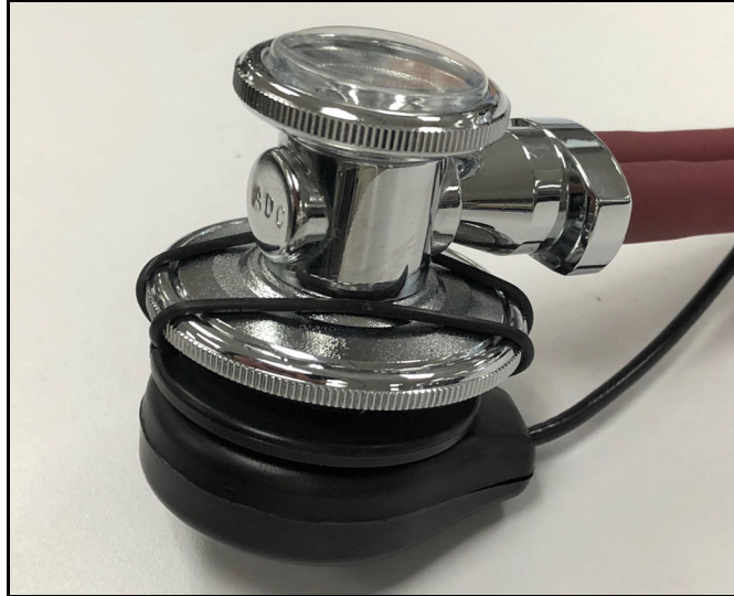
StethoSym Speaker Module Connected to Diaphragm
