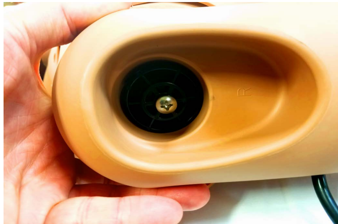
NIBP Arm Attached and Ready for Pad Installation
