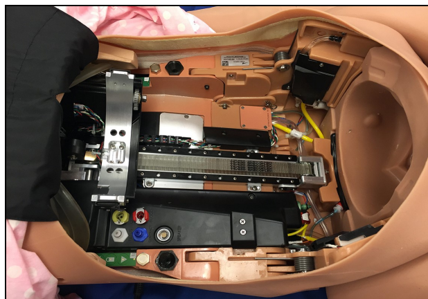
The Manikin's Torso - Rotation Ring Removed
