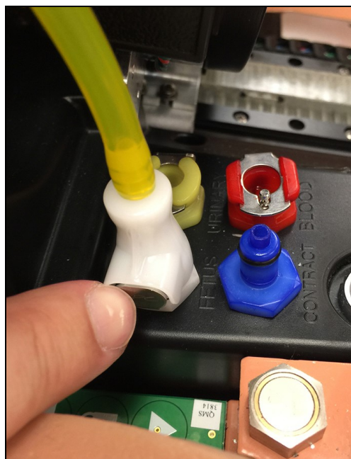
The Manikin's Torso - Rotation Ring Compressor Connection
